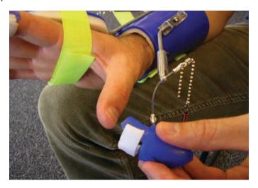
3. Re-attach the Spring to the Thumb Lead Mount.
