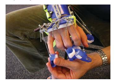
7. Locate the Spring and re-attach it onto the Hook on the Wrist Mount located on the Forearm Shell.
